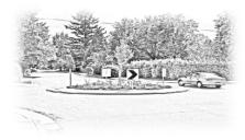
Traffic Circles are raised islands, placed in intersections, around which traffic circulates. They are designed according to the existing geometry of each intersection and sized to accommodate the passage of an emergency vehicle.
